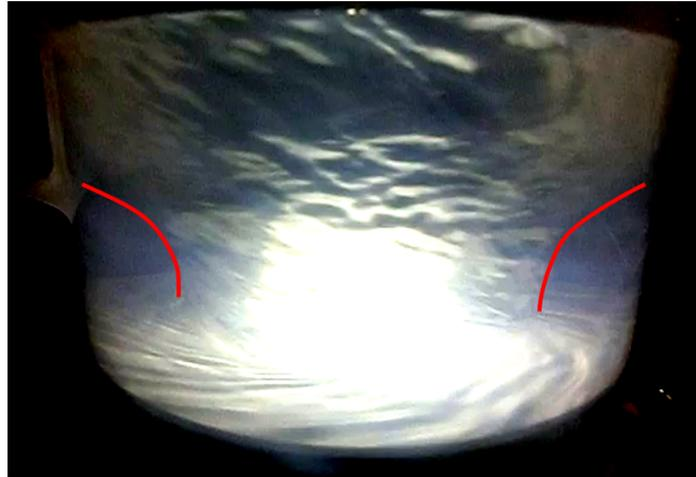
**Fig. 7:** Side view of the fluid surface in the axisymmetric state, with the fluid surface traced by the red curves.
