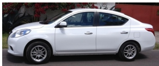
Figure 1. Test car, automatic, gasoline, 4-cylinders, 106 HP, size of 1.6 L.
